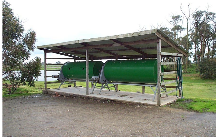
Figure 3: A typical rotary composter used in the Australian poultry industry (VFF 2001).
