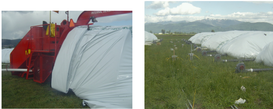
Figure 4: Ag-Bag ® in-vessel composting system in use in Canada (DAFF 2005).
